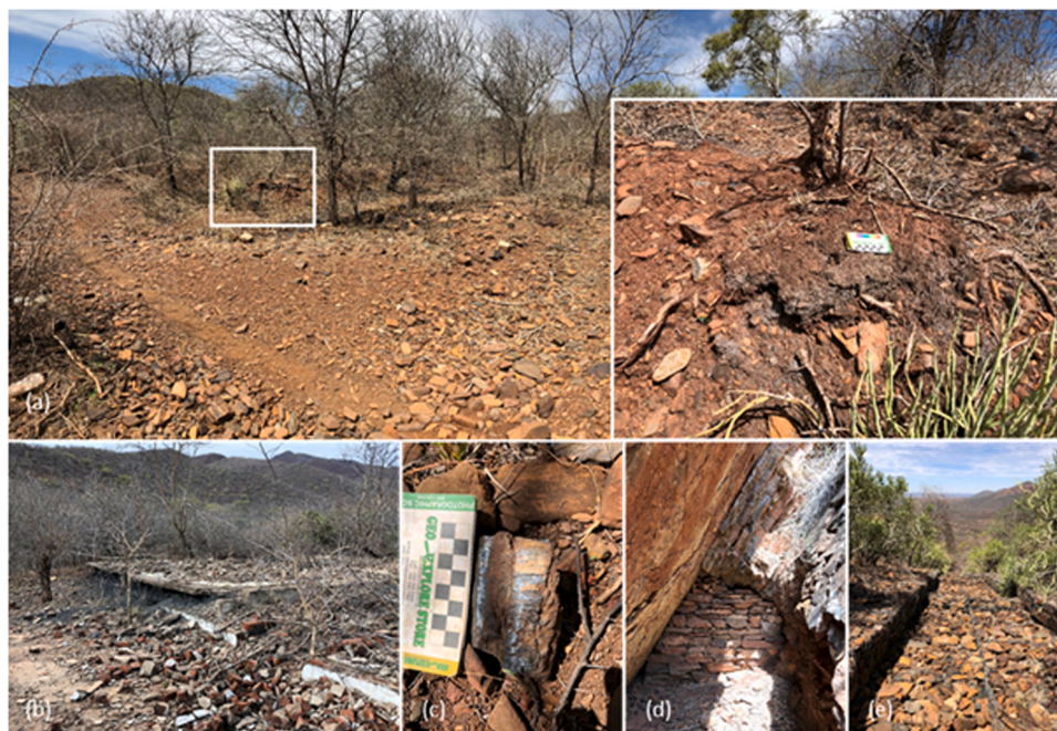
Fig. 4. Observations at the Uitkyk mine site. (a) The Uitkyk mine is immediately adjacent to the Lagerdraai mine; view looks eastward toward Uitkyk. The alluvium in the valley is extensively polluted with processed asbestos waste; (inset) caked processed asbestos fibres at the site, sample U21. (b) Old mine housing foundation slabs, with asbestos fill, eastern part of Uitkyk, sample U17. (c) Waste rock with asbestos ore, near the head of the valley at Uitkyk, sample U02. (d) Old mine offices foundation slab; the area is near a site of processed asbestos, 200 m east of the river. (e) Process material remnants, cut by E to W erosion that drains to the Tlhabosane River.
